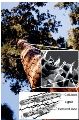
Wood as an example of a natural lightweight nanocomposite for large structures. It exhibits a hierarchical architecture and sophisticated structure on the nanometre scale. © BOKU Vienna
