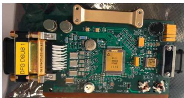
Flight Model of DFG electronics with Magnetometer Front-end ASIC in the middle (chip with golden lid). © ÖAW/IWF
