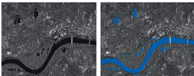
RAPIDEM prototype results of near real-time TerraSAR-X based water body detection. © GeoVille
