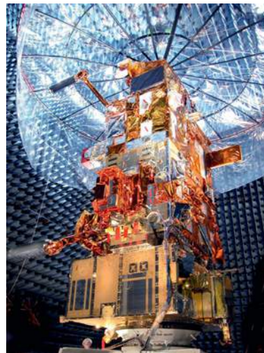
MetOp spacecraft during testing. © ESA
