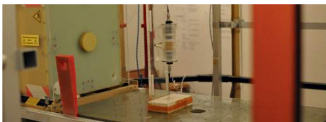
Calibration of the CDSM sensor in the Braunkerk coil facility of TU Braunschweig, Germany. © ÖAW/IWF
