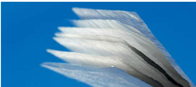
Super-insulation for cryogenic applications. © RUAG Space GmbH
