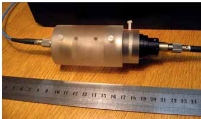
Current CDSM sensor unit (TRL 3 standard)
