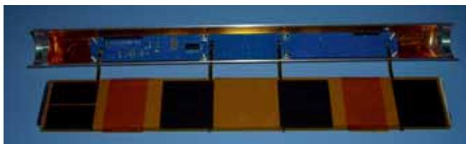
The PP instrument during an integration test for the HP3 ESA preliminary design review (PDR). The HP3 instrument was rated by ESA as TRL 5 during that review.
