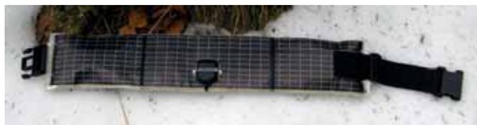
Telemetry test collar with solar panel and GPS antenna
