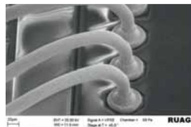
Electron microscope image of bonding detail.
