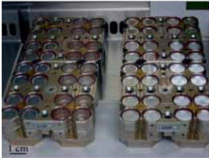
Sample holders of the ISS experiments ADAPT (left) and PROTECT (right) following dismantling in a work bench. Crystals of halite on quartz discs attached with red glue are visible in the left tray.
