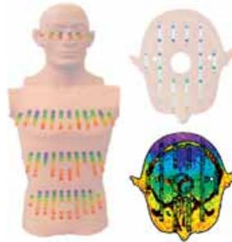
Figure 2: Experimental TLD results of the depth dose distribution due to frontal photon exposure of the MATROSHKA phantom (left and right top) and comparison with simulation results (right bottom).
